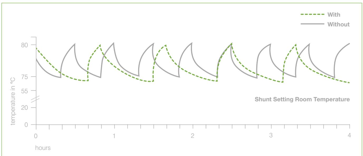
The boiler's cycles over a 4 hour period are reduced from 8 to 5, and the overall 'burn' time is reduced from 80 to 62 minutes.
