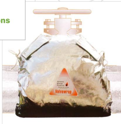
a casing consisting of an outer cover of Aramid cloth with a triple-coated polymer aluminised coating. Each wrap has an inner cover of woven Aramid cloth with an internal silicon coating.
